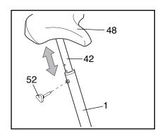
dismount the exercise cycle, hold the Seat and remove the Seat Knob (52). Raise or lower the Seat and reinsert the Seat Knob. CAUTION: Make sure to insert the Seat Knob through the welded nut on the Frame (1) and the Seat Post (42); do not insert the Seat Knob under the Seat Post.
